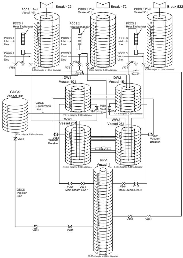
Figure 3: TRACE Nodalization of PANDA Facility
